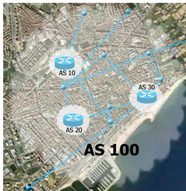
Figure 6.2: Configuration of BGP confederation in the selected area
