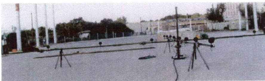
Figure 1: The Rafael Helispot system is an example of modern tactical use of sonic information. The microphone array has demonstrated the ability to detect and classify helicopters at ranges of a few Km, at acoustic frequencies.
